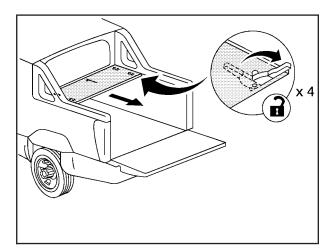
Remove cargo panel 1 (if you need to), but notice that there are four latches to release (two left-side latches and two right-side latches). Set the panel aside.
